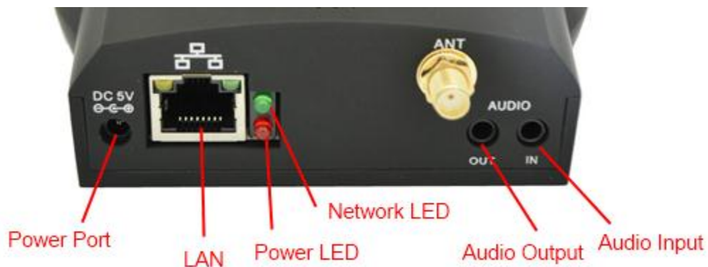
Figure 3.2 – The rear of the FI8910W. Includes a DC 5V/2A power supply port, RJ-45/10-100 Base T port, power and network lights, and input/output audio jacks for external speakers or microphone
