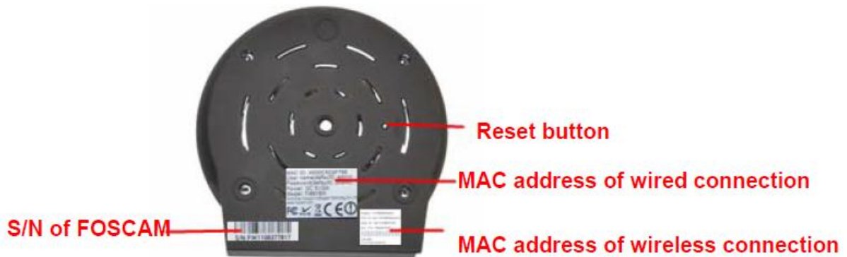
Figure 3.3 – The bottom of the camera shows the wired/wireless MAC addresses of the camera. It also shows the S/N number and has a reset button.
